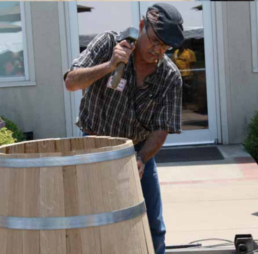
Top left: The first ring is put in place. Middle-left: The second ring is positioned with a hammer and wedge. Bottom-left: The barrel is thoroughly heated. Top-right: The cable is tightened around the opposite end. Bottom-right: The bottom two rings are installed and the barrel is ready for the final toast
