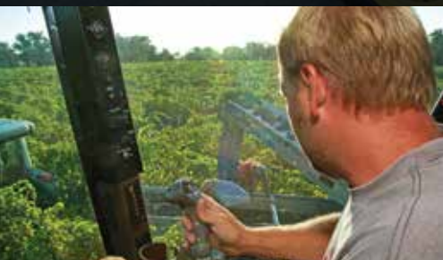
Adam Nunnikhoven controls his speed carefully to maintain the conveyor's position above the receiving bin.
