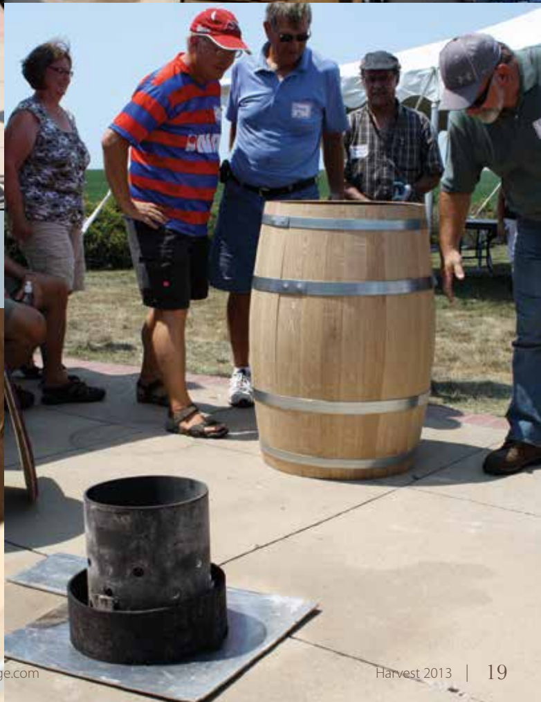
Top left: The first ring is put in place. Middle-left: The second ring is positioned with a hammer and wedge. Bottom-left: The barrel is thoroughly heated. Top-right: The cable is tightened around the opposite end. Bottom-right: The bottom two rings are installed and the barrel is ready for the final toast
