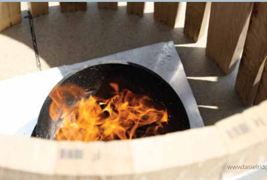
Top left: The first ring is put in place. Middle-left: The second ring is positioned with a hammer and wedge. Bottom-left: The barrel is thoroughly heated. Top-right: The cable is tightened around the opposite end. Bottom-right: The bottom two rings are installed and the barrel is ready for the final toast
