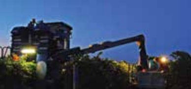
Harvested grapes are conveyed to Macrobins travelling on a cart in the next row.
