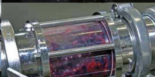
Must is visible through a sight glass.
