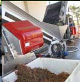
The destemmer separates the rachis from the individual grapes.
