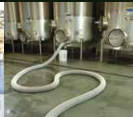
The "must" (crushed grapes, juice, skins, and seeds) is pumped into a tank.
