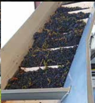
The elevator carries the grapes up above the destemmer-crusher.
