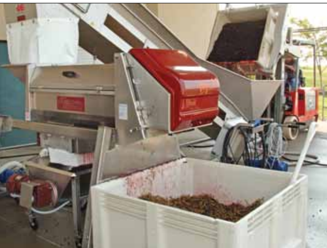
Top: Brock drives the Korvan as it harvests Marquette. Top-left: Marquette harvesting started before daybreak. Top-right: Denise and Amber removing MOG (material other than grapes) from bins on trailer. Bottom-left: Elevator, destemmer-crusher, and must pump process the fruit and send it to the tank for fermentation. Bottom-right: Jonita starts the elevator as grapes are dumped from the bin.
